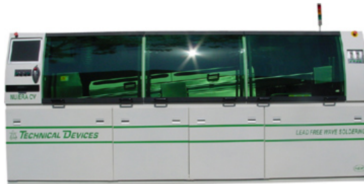
18-Inch Process Width Computer Controlled Wave Soldering Machine (actual machine may vary from picture above)
