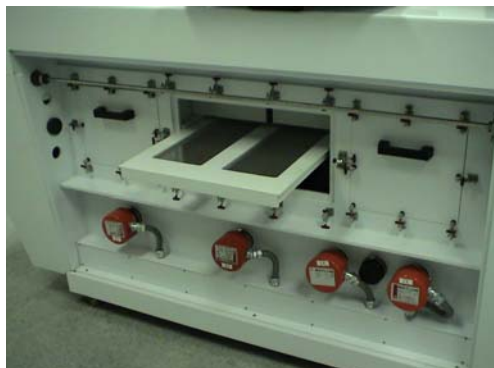
Easily Accessible Immersion Heaters and Catch Screens (Shown with Front Panel Removed)
